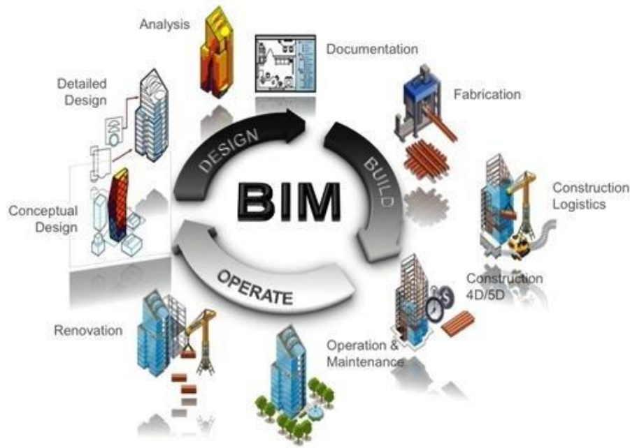
Figure 2 Life cycle of a 3D building model; source: (Logothetis et al. 2016)
