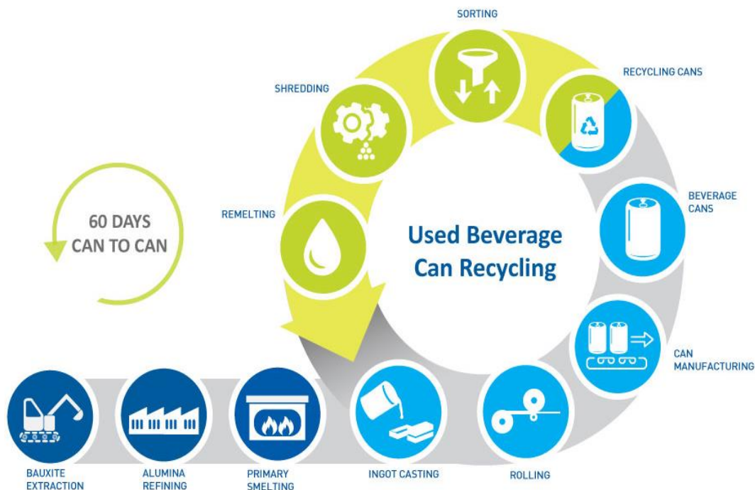
Figure 4 The aluminium beverage cans manufacturing diagram; source: modified by (Farner, 2000)
