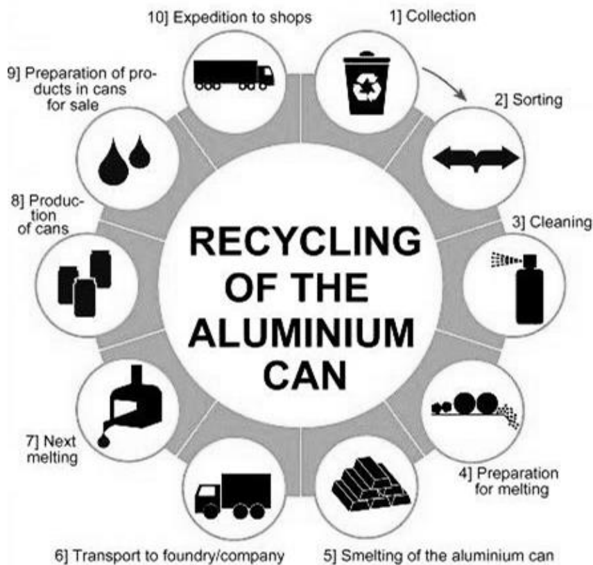
Figure 5 Recycling process of the aluminium can; source: modified by (Farner, 2000)
